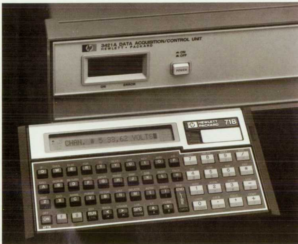
Fig. 1. The HP 82479A Data Acquisition Pac for the HP-71B Computer enables the computer to control the HP 3421A Data Acquisition/Control Unit via the Hewlett-Packard Interface Loop, allowing an engineer to configure low-cost, battery-powered systems for data logging or instrument control.
